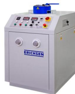
Universal Sheet Metal Testing Machine with Automatic Test Sequence - Model 142
