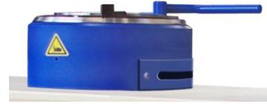
All components are easily accessible from outside the machine, and thus the tools for the individual tests can be changed quickly, too. The operator's controls are well arranged on the control panel. The operating sequence of the testing machine has been designed in such a comfortable manner that cutting of the blank as well as drawing and ejecting of the cup are executed in one single operation.
