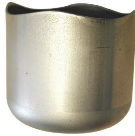
Deep Drawing Cup Test
