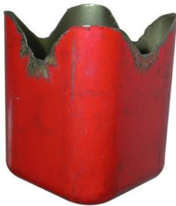
Square Deep Drawing Cup Test
